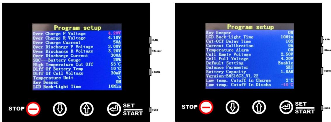
13. Set balance is on, please check if the cell voltage difference is going down, for over 50AH battery, the changes are very slow. But if the main unit case is warm, it means the cells are balancing. Adding a cooling fan to the main unit can speed up the balancing.
