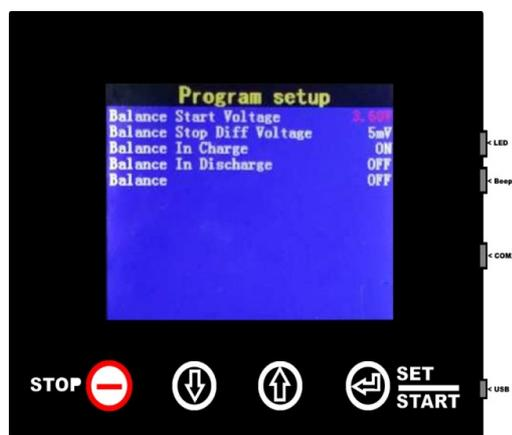
14. Set accurate battery capacity, then charge or discharge the battery, the charged or discharged capacity must be 25% of battery capacity setting at least. The SOC will be calibrated automatically.
