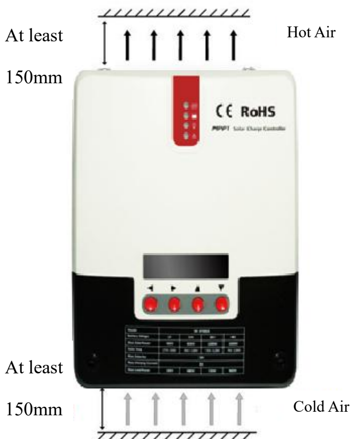
Figure 2.1 Installation and Heat Dissipation
