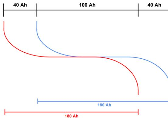
3. A correction drift may occur if the capacity of the cells has changed due to cold temperatures. Some cells (notably iron-phosphate cells) have a restricted range in the cold which can be as little as 50% of the normal capacity.
